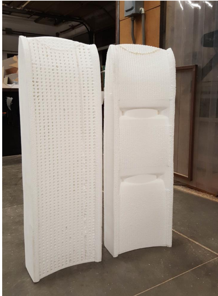
Figure 44 The final physical model for the wind tunnel test. (Photo by author)
