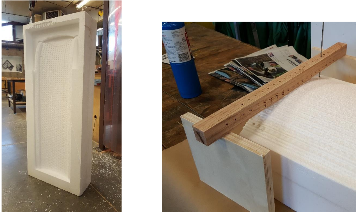
Figure 41 The physical model made by CNC machine on the left and creating the penetration on the model on the left. (Photo by author)
