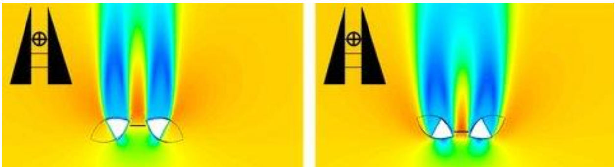
Figure 22 Results of computer simulations on the two configurations of the Bahrain WTC. The left picture shows the current configuration of the two towers, the right picture the situations in which the towers are built the other way round. The colors indicate the wind strength and the wind direction is up. The horizontal line between the towers indicates the position of the wind turbines. It is clear that on the right picture the area around the line is more red, indicating stronger wind flows. [111]
