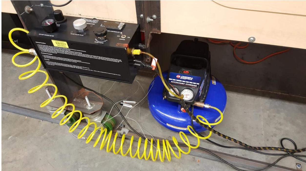
Figure 45 The compressor pressure 20 psi. (Photo by author)
