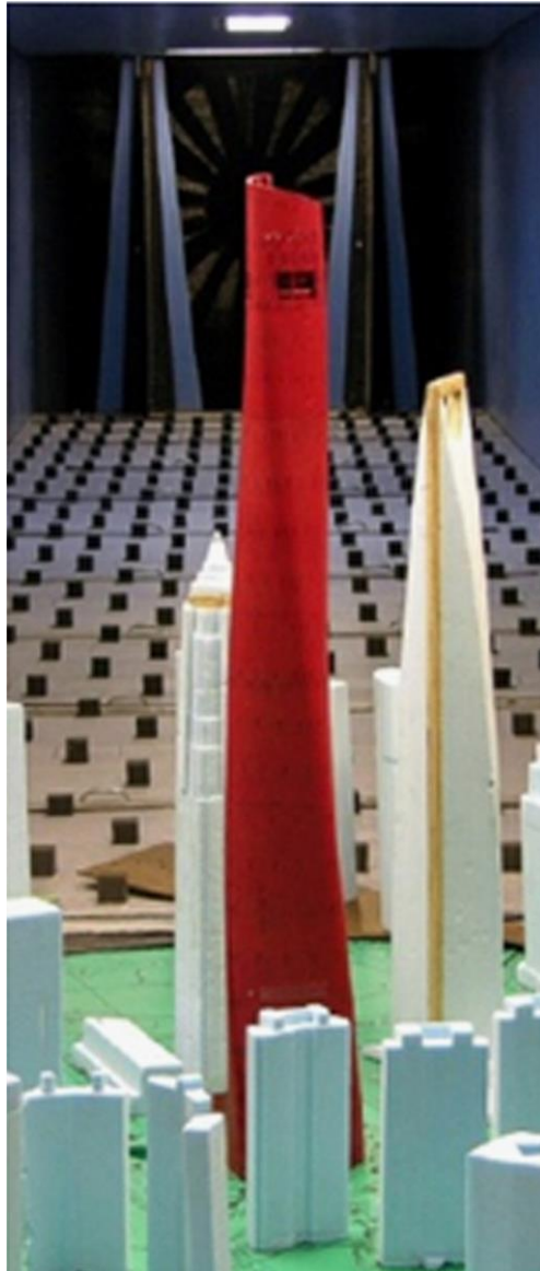
Figure 9 Shanghai Tower, twisting and tapering modification.[52]
