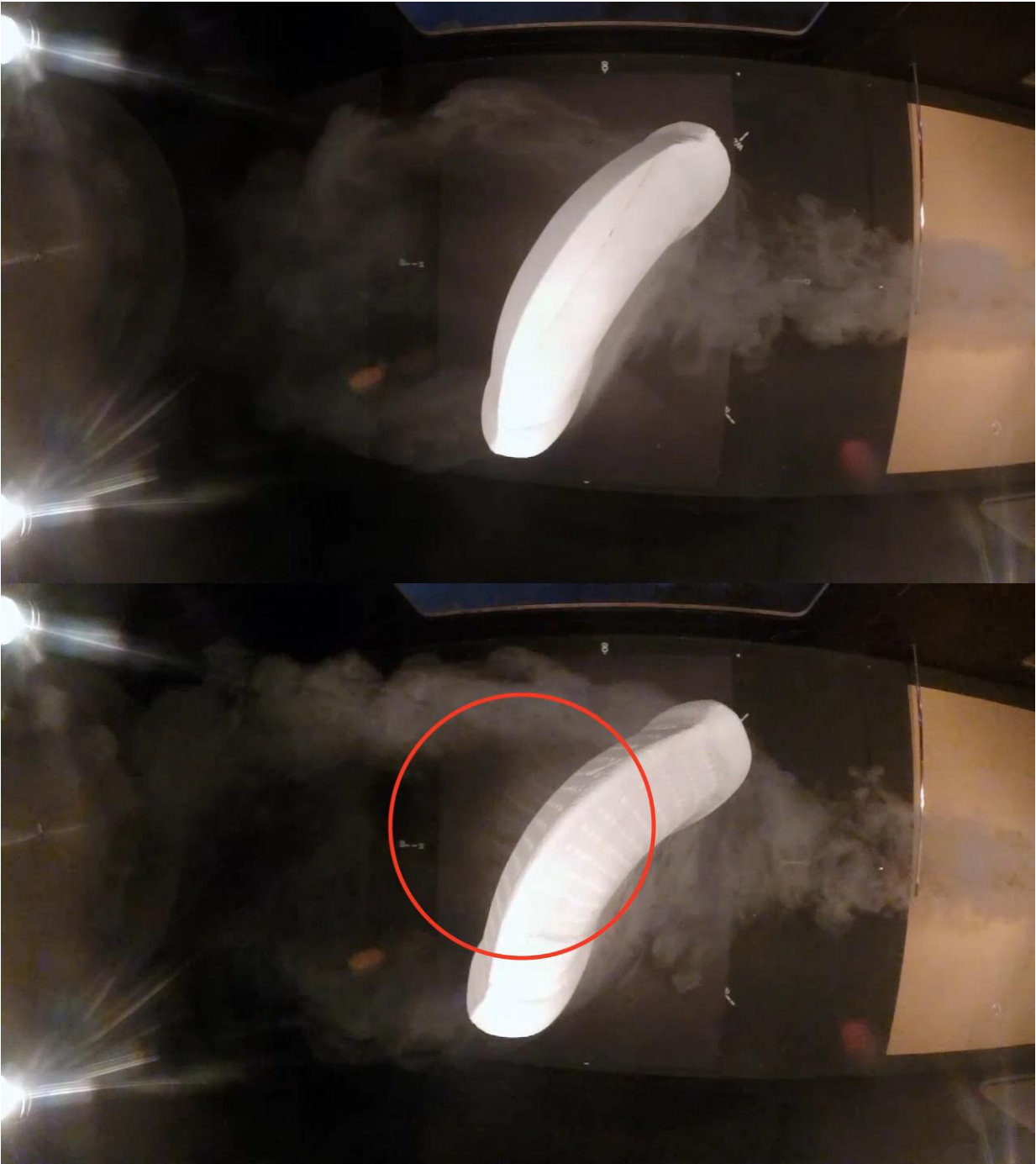
Figure 53Original building on top vs proposal idea on bottom. The wind passing capacity for the angular wind. (Photo by author)
