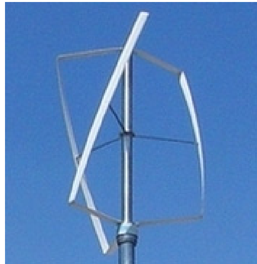
Figure 2: Turby Vertical Axis Twisted H-Darrieus Wind Turbine
