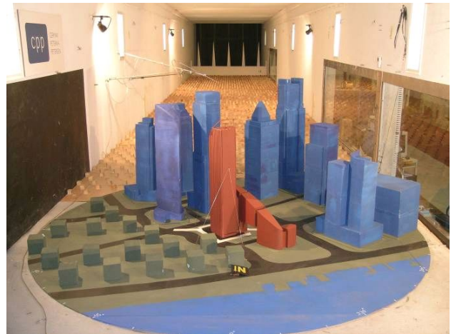
Figure 12: Photograph of a scale model installed in an atmospheric boundary layer wind tunnel to evaluate the potential for building integrated wind turbines.
