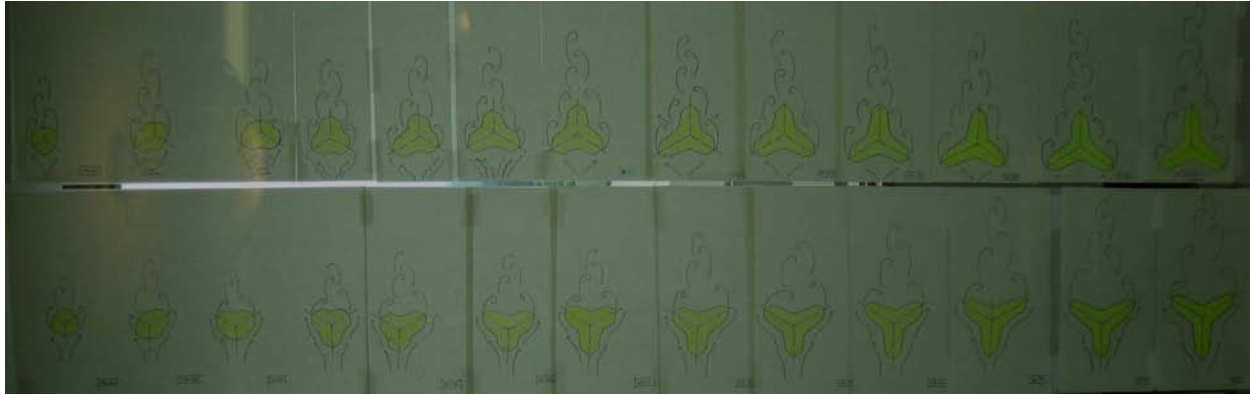
FIGURE 3- WIND FLOW VARIATION AROUND AND ALONG THE HEIGHT OF THE TOWER
