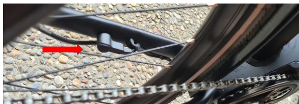
Fig. 3 Demonter original hastighetssensor
