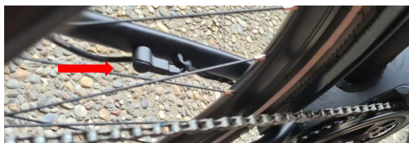
Fig. 3: Demonter original hastighetssensor
