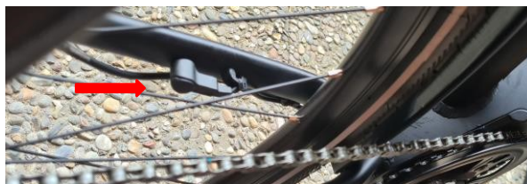
Fig. 3 Demonter original hastighetssensor
