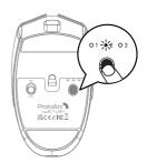
2. Press the mode switch button and switch to 2 or 3 mode, the white light flashes slowly.
