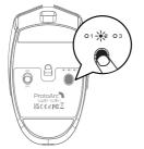
3. Press and hold the mode switch button for 3~5 seconds until the white light flashes quickly, then the mouse enters the Bluetooth pairing mode.
