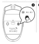
3. Press the mode switch button until the white light 1 is on and enter 2.4G mode
