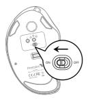
Turn on the power switch to ON.
