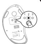
3. Press and hold the mode switch button for 3–5 seconds until the white light flashes quickly, then the mouse enters the Bluetooth pairing mode.
