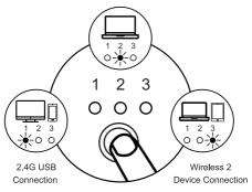
Press the mode switch button on the top of the mouse to switch between 3 devices.
