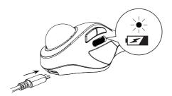
Plug the charging cable into the USB port of the computer. The charging light will turn red during the charging process. The charging time is about 1-3.5 hours. The charging light will turn green after the charging is completed.
