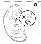
3. Press the mode switch button until the white light ① is on and enter 2.4G mode.
