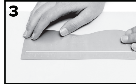
Align the Ruler Stencil to cut in a straight line and desired length
