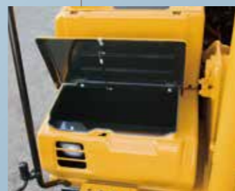
▲ Large capacity toolbox equipped with air pressure spring
