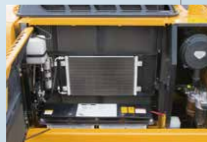
▲ Cooler The oil cooler and the intercooler and the radiator are arranged parallel to make the cooling effect better.
