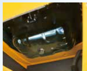
▲ The fuel tank is equipped with a discharge cock
