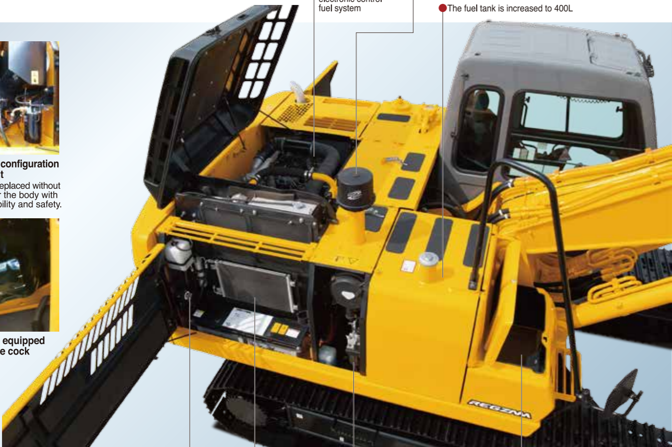
▲ New air pre-filter that does not require the special maintenance
