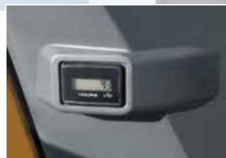
▲ Hour meter The location of hour meter is improved so as to confirm conveniently from outside of the cab.
