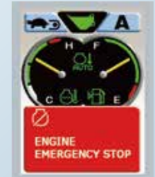
◀ When engine emergency stop switch is operated
