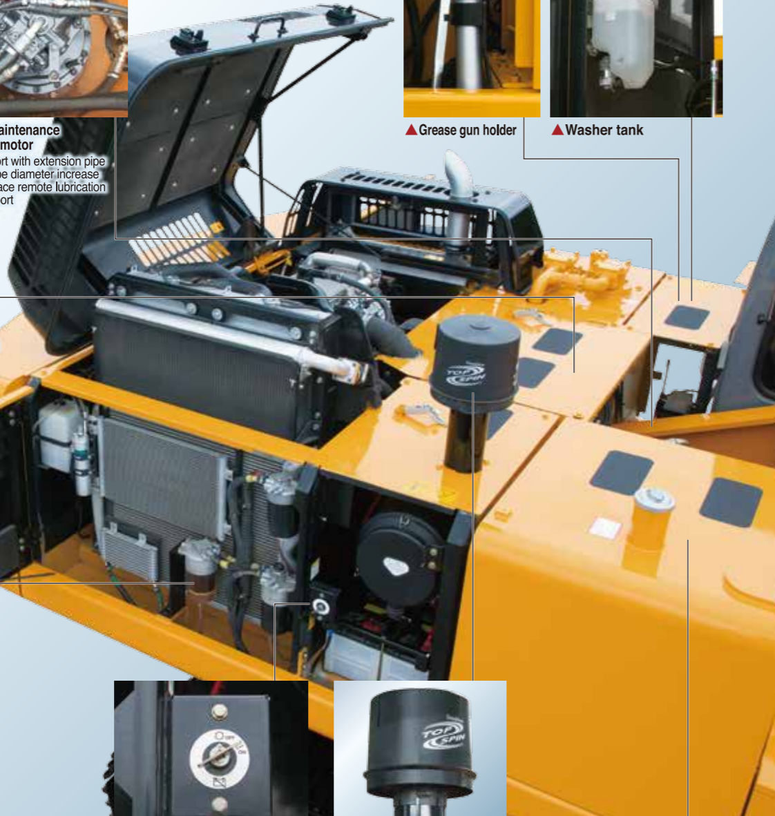
▲ Equipped with battery disconnect switch
