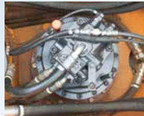
▲ Easier maintenance of swing motor ● Filling port with extension pipe ● Drain pipe diameter increase ● Top surface remote lubrication grease port
