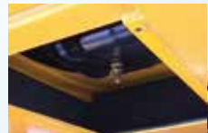
▲ The fuel tank is equipped with a discharge cock
