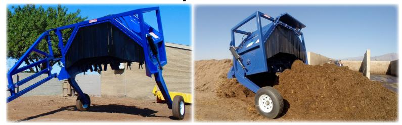
Foldable side bar for compact storage and/or transport: Length 4.42 m | Width 2.903 m | Height 1.902 m
