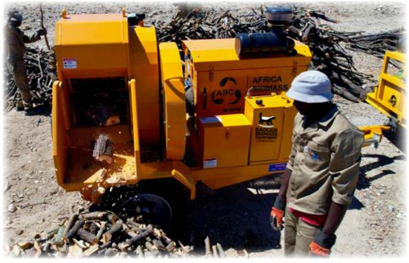
The hydraulics of the machine is also capable of powering a stacking conveyor (on a separate trailer) to load the billets up to 3.6 m high.
