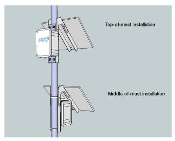
When the unit is mounted on the top of a mast longer than 3m, the brackets can be moved around to ensure even weight distribution.
