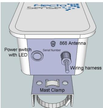
• Before switching the unit on, ensure that you have connected the antenna.
