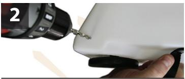
Drill the 1/4" hole on bottom left corner of the side with the cord connection 1/2" from bottom of sign.
