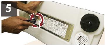
Use Phillips head to screw bottom plate light panel back into place.
