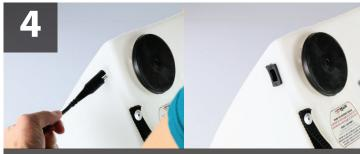
Insert new pigtail into hole and push it into place. This might require a bit of force.
