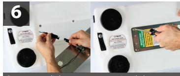
Connect new light system to new pigtail, then screw plate back into place with screwdriver.
