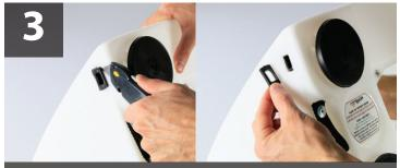
Use razor to cut around the outer edge of the old pigtail socket. Remove through bottom of sign.
