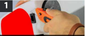
Using a sharp blade, cut pigtail lip off of topper. Always cut away from your body to avoid injury.
