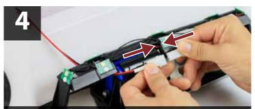
Plug in new pigtail into new light system. Discard old light system.
