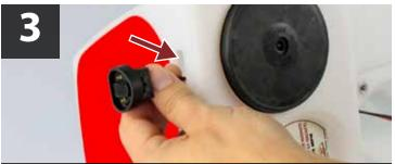
Feed magnetic pigtail into hole and use hand to secure into place. This may require a bit of force.
