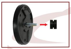
Push rubber grommet onto magnet screw.
