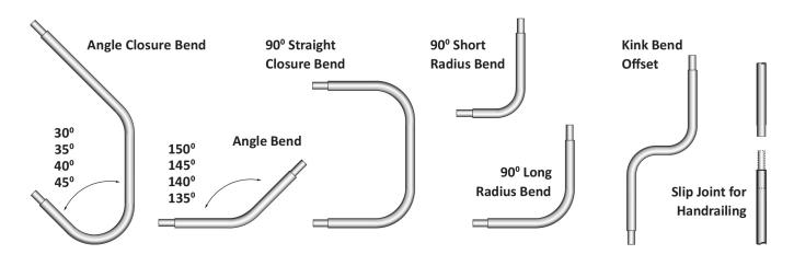
Handrail Stanchions and Accessories are supplied in Mild Steel, Zinc Chromate, Galvanised, 3cr12, Stainless Steel, Solid Forged and Fibreglass.
