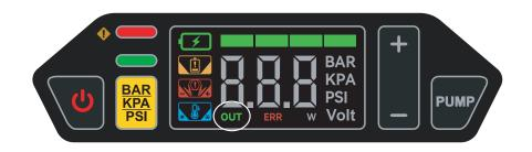
You will need the following: USB-A To USB-C cable and a mobile phone (if the mobile phone supports 9V2A of QC protocol, it can support 9V2A fast charge) Connect the A port of the USB cable to the product and the C port to the Type-c charging port of the phone, and the "OUT icon" of the product will start charging.
