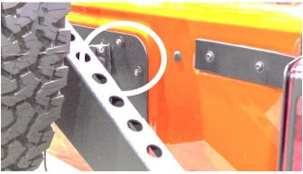
With the mount in hand turn and place the two beveled bolt holes up to the tailgate holes. Using the included hardware and a 13mm socket or wrench, secure the mount into your tailgate. Be sure to not over tighten as it may damage your body.
