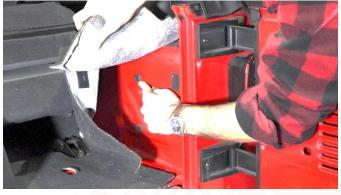
Remove this plug, and with a utility knife, cut the point off until it is large enough to pass the Backside's wiring through
