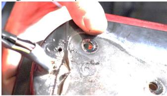
Push both ground wires through the hole, and begin reinstalling the taillight. Loosely secure the bolt nearest to the wires, and coil the wire around the stud. Secure them into place by tightening the bolt down onto the wires, creating a ground.
