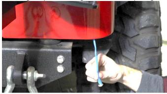
Before cutting any wires, be sure there is enough slack in the wire for the tailgate to open and close comfortably, and without it getting pinched in the door.
