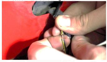
Wrap the Backside wires around their respective taillight wire, and secure them with electrical tape or your preferred method. Remember not to secure the black wires at this time.
