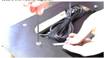
Next, install your license plate using the (4) % -20 bolts and flange nuts with a 4mm Allen and 11mm wrench.
