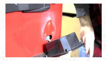
Reach under the tub, below the passenger taillight, and pull down the wire that was pushed through the interior. Open the tailgate completely to allow the wire to set its optimal length.
