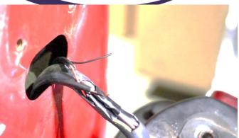
Begin grounding the Backside wires by drilling into the back of the taillight case. With a 1/16" drill bit, drill a small hole just below either the left or right bolt hole, as shown. Be careful not damage the wiring, bolt holes, or lamps.
