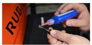
Completely unscrew the adjustment bolt, removing the top portion of the latch. Apply threadlocker to the threads \*.
