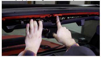
With a T25 Torx bit, unscrew and remove the footman loop, save factory bolts for future use if needed.
