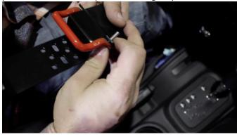
Insert the included bolts through the front and begin securing the mount and footman loop back into the windshield frame, using a Philips screwdriver.
