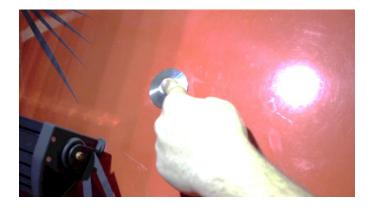
With the other, secure a washer and a nut to the countersunk bolt. With a 13mm socket and 5mm hex wrench, tighten the nut and repeat on the opposite side.
