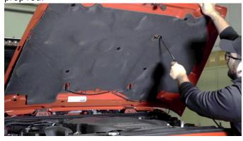
Peel back the heat shield enough to gain access the hood bumper nuts.
