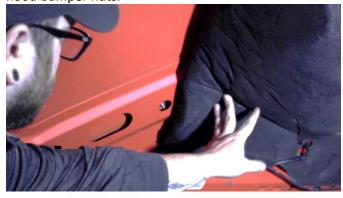
On a JK, with a 10mm socket, hold the bumper with one hand and unscrew and remove the nut. Repeat on the opposite side.
