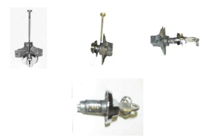
Place a very small screwdriver in the square hole at the top of the key lock mechanism. Push down on the retaining clip while pulling on the cylinder of the key lock. Once the cylinder is loose put the key in to prevent the tumblers from falling out. To reinstall the key lock, with the key in the cylinder slide the tumbler into the housing and remove the key.
