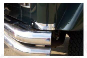
Align the bottom edge of the guard with the body tub. Mark the two mounting holes with a permeant marker. Center punch the mark, then drill a pilot hole with an 1/8" drill bit. Re-drill the holes using an 11/32" drill bit. Bolt the corner guards in place using the stainless-steel bolts provided.
