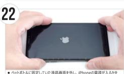
確認します。確認後は必ず電源をOFFにし、手順20と21で取り付けた 4か所のコネクタを全て外して、液晶画面とバッテリーを取り外します。 Remove and lower the screen from the drinks bottle and test whether the iPhone can be turned on with the new battery. After confirming the phone can be turned on, turn off the power and reattach the screen with the rubber band and remove the battery. If it cannot be turned on, please check wether the battery cable is properly attached. 将屏幕从固定位置取下,测试iPhone是否能开机,确认可以后请关闭电源并重新用 橡皮筋将屏幕固定,再将电池拆下。如果不能开机,请重新检查电池排线是否扣好。
