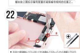
イバーを使用し、(16・17・18) 番で取り外したバイブレーターを逆の手順で取り付けます。 Use tweezers to place the metal part (C), and use the Phillips screwdriver to lock in the screws (found on the magnetic pad in the position corresponding to the number shown above). Use your fingers to attach the cable. When the cable is attached, a "click" sound is heard indicating the cable has successfully been attached.
