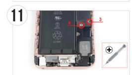
Use the Phillips screwdriver to unscrew the screws counterclockwise as circled above. Place the removed screws onto the magnetic pad in the position corresponding to the numbers shown above. 用十字螺丝刀在上图圆圈外沿逆时针方向将螺丝旋开 螺丝按上图标示编号放置在磁垫编号相同的位置上。
