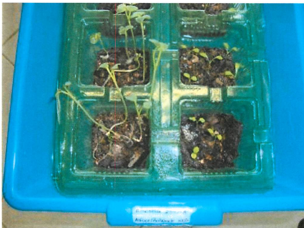
Figure 18: Radish (left) and lettuce (right) germinated and grown in the organic compost containing LDPE + PDQ-H (Sample 2343) obtained from the degradation test.
