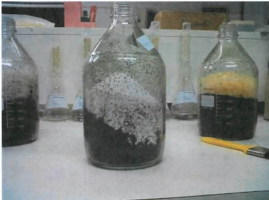
Figure 5: Flasks containing 100g of microcrystalline cellulose (Positive Control) and 600g of organic compound.
