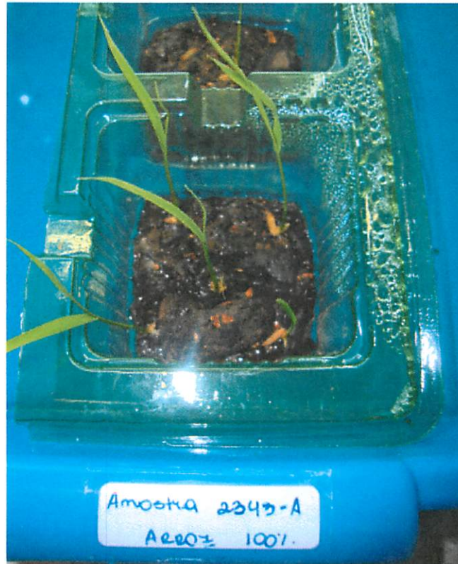
Figure 20: Rice germinated and grown in the organic compost containing LDPE + PDQ-H (Sample 2343) obtained from the degradation test.
