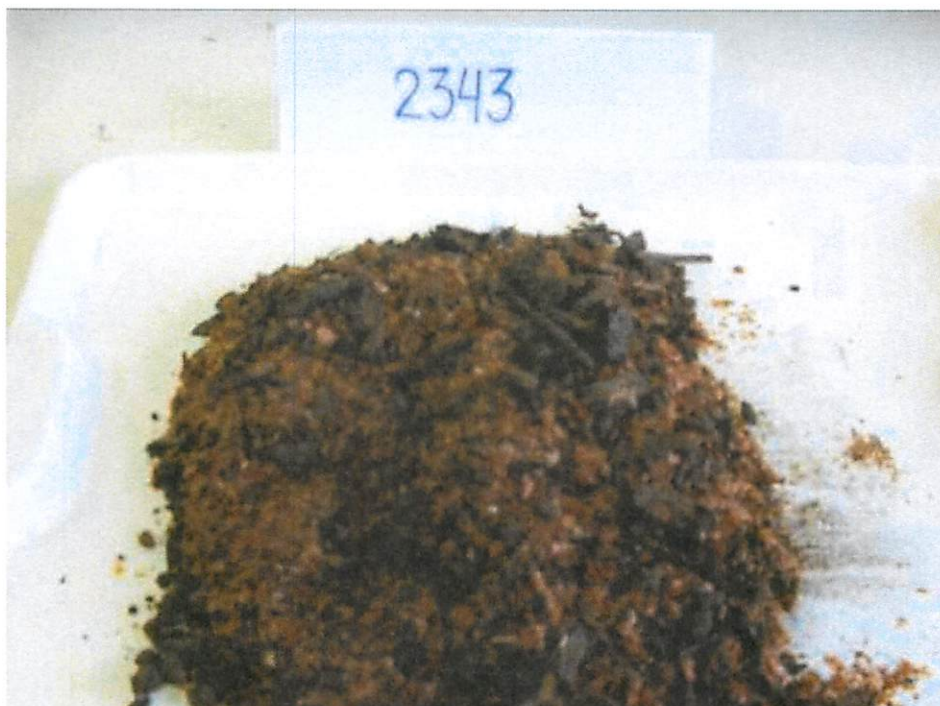
Figure 10: General appearance of the compost containing PDQ-H + LDPE (Sample 2343) after 121 days of exposure.
