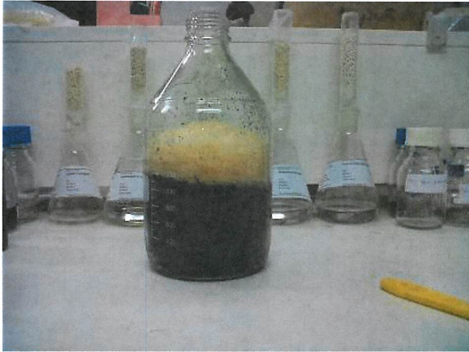
Figure 4: Flasks containing 100 g of LDPE + PDQ-H (Sample 2343) and 600g of organic compost.
