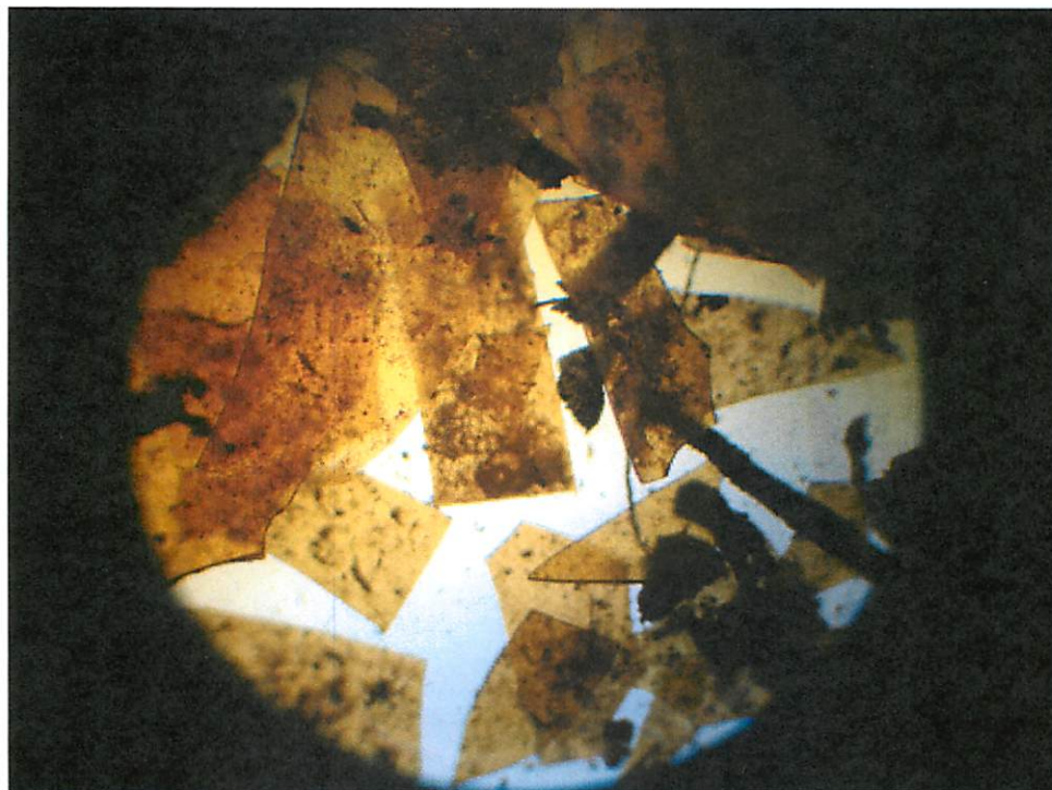
Figure 12: View of the sample LDPE + PDQ-H under microscope (40x magnification). Appearance after 121 days of exposure.
