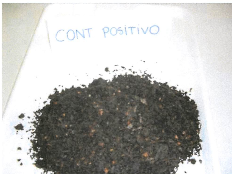
Figure 9: General appearance of compost containing cellulose (Positive Control) after 121 days of exposure.
