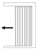
Slide the free end "I" section of the panel directly into the cabinet. Slide the panel down. Be sure to leave enough space to slip the top and bottom of the frame into the rails on the cabinet.
