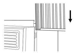
Once the panel has been installed on the side of the cabinet, make sure it sits securely inside the frame channel by making slight adjustments. Slide the top and bottom ends of the frame into the top and bottom rails of the cabinet.
