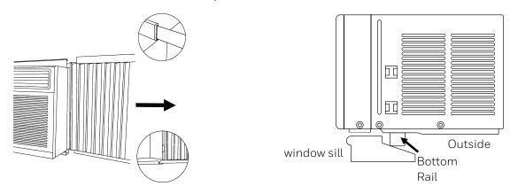
Once the air conditioner is placed, extend both the left and right accordion panels to the width of the window.
