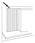
To secure the lower sash into place, use the sash lock and a 3/4" screw as shown below.
