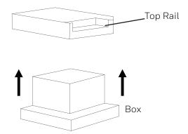
**02** Secure the top rail to the unit with the 3/8" screws
