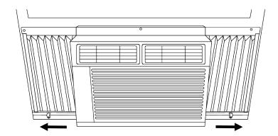
**02** Place the frame lock between the extended accordionpanels and the window sill. Screw a 3/4" (19mm) locking screw through the frame lock anc into the window sill.
