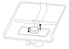
02 Rotate the filter insert counterclockwise to unfasten and detach the filter insert.
