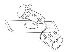
**05** Reassemble the filters in the reverse order of the dissasembly, replace the filter insert, and rotate clockwise to the close arrow.
