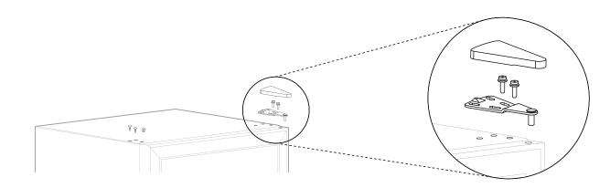
**05** Put the glass door on the lower hinge, install the door axle sleeve back and then install the upper hinge. Align the door with the cabinet and check the tightness of gasket.
