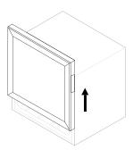
**02** Open the door of the beverage cabinet and detach the glass door with tremendous care.
