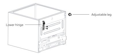
**06 06** Put the door on lower hinge vertically, then install the upper hinge by fitting screws and the hinge cover. Cover the hole caps on upper right side.
