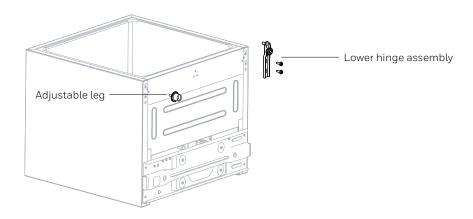
Install the lower hinge and adjustable leg on lower left side of cabinet and lower right side respectively;
