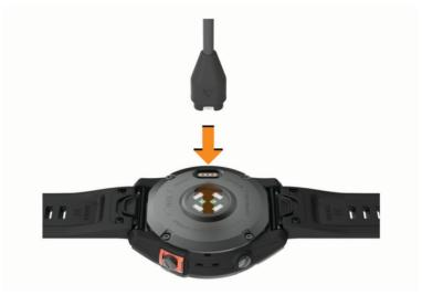
2 Plug the other end of the cable into a USB charging port. The watch displays the current battery charge level.
