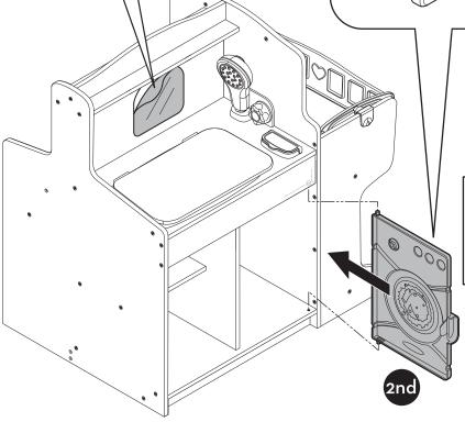
IMPORTANT: Insert the top hinge pin first, then flex lower hinge pin to insert.
