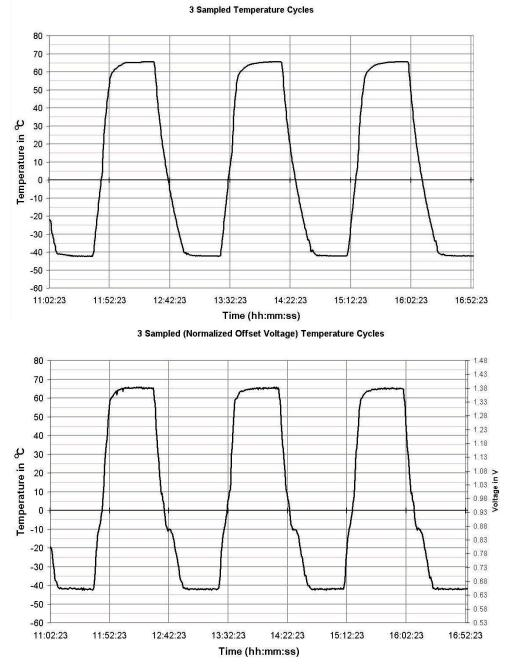
\*The above chart includes the analog offset voltage of one test unit to confirm that units in the test chamber reached the desired temperatures at the same time as the chamber. Offset voltage is normalized using the equation below.
