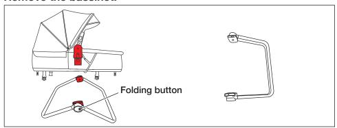
Remove Hatch™ Bassinet mattress and waterproof sheet or changing pad, whichever is being used. Press the reversing button on both sides of the bassinet to take the support frame out. To fold the support frame, press the folding button on both sides of the support frame and collapse into a folded position.
