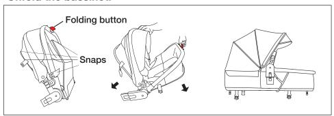
Once the bassinet is securely in frame, unhook all snaps if needed. Lift the folding buttons up to release the lock, then open up the bassinet until hearing a clear "click" sound. Attach the handlebar. Put Hatch™ Bassinet mattress with waterproof sheet on (sold separately). Use changing pad as needed.
