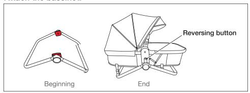
Open the support frame and put it on the ground. Make the reversing button perpendicular to the bassinet pocket, then attach the folded bassinet to the support frame connecting part by pushing down until hearing a clear "click" sound then proceed with unfolding the bassinet.
