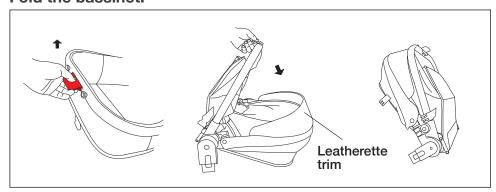
Lift the folding buttons up to release the lock, tuck the leatherette trim in, then fold the bassinet and attach the snaps by the folding buttons.
