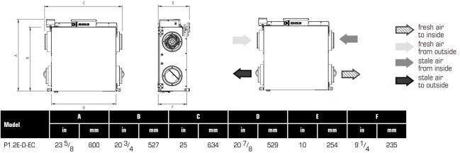
Clearance of 8.5 in. (216mm) in front of the appliance is recommended for removal of core. All appliances feature three foot plug-in power cord with 3-prong plug.
