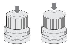
6. Install the top cover by aligning the top cover notch and lever position.
