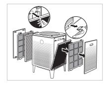
2. Remove the plastic wrapping for the new Max2 filters and discard it.
