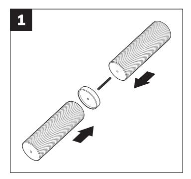
Screw threaded rod **D** into posts **A**, through center ring **B**.
