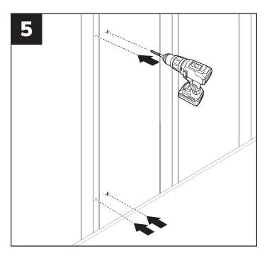
Drill two holes through the drywall using a ½" drill bit, and two additional pilot holes straight into the wall studs using a ½" drill bit.
