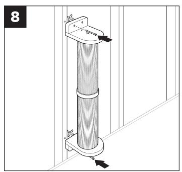
Drive mounting screws **H** straight into the pilot holes and stud.
