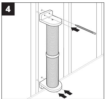
Use a pencil to mark the locations of all four holes you'll be making. Make sure that two holes align with the wall stud.
