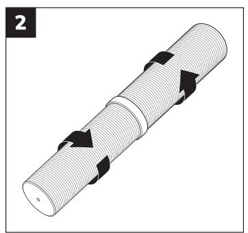
Twist posts clockwise until they are tightly pressed together against the center ring.
