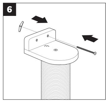
Separate toggles from toggle bolts **G**. Insert bolts through the holes of the mounting plates and reattach toggles.
