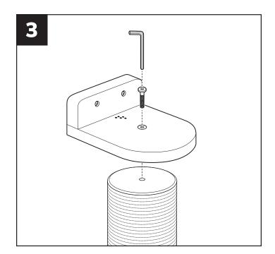
Fasten hex bolt **E** into mounting bracket **C** using hex key **F** on both sides.
