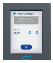
Set your **Outflow Height**, this is the height that water is drained from your tank, normally around 0.1m.
