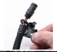
5. Pull the wiring loom away from the wires.
