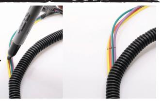
**7.** Pick **ONE** of the wires to start with. Cut it and move on to step 8.
