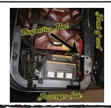
**4.** If you have wiring loom covering the wires leading to the data port, remove it by peeling back the electrical tape holding it in place.
