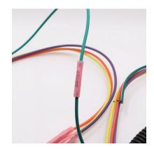
**10.** Crimp the connector. Go back to step 7 and repeat the steps until all four wires are connected.
