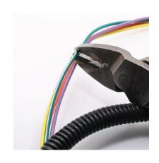
**8.** Strip the wire you just cut on the side leading to the controller.
