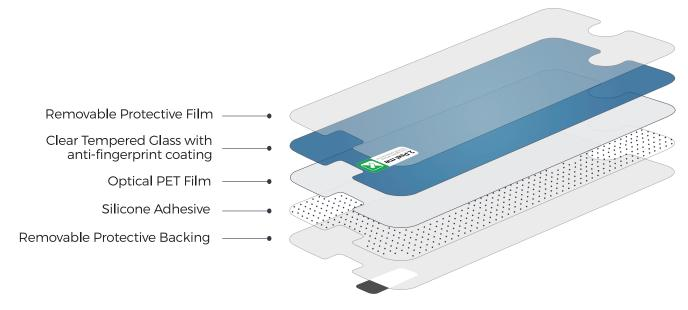
Optic+ Nano-Glass screen protectors are made up of a number of layers. The Multi-layered Nano-Glass provides a high level of flexibility which in turn improves impact resistance and removes the risk of shatters and sharp glass shards.
