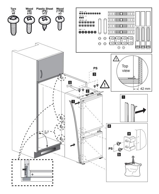
**Note:** Installation step for 2, screws for connecting top plastic part should not be screwed very hard, because of moving the plastic part easily left or right side.
