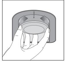
Operating temperatures are controlled by the thermostat knob (see diagram) located on the ceiling of fridge compartment. Settings may be made from 1 to 5, 5 being the coldest position.
