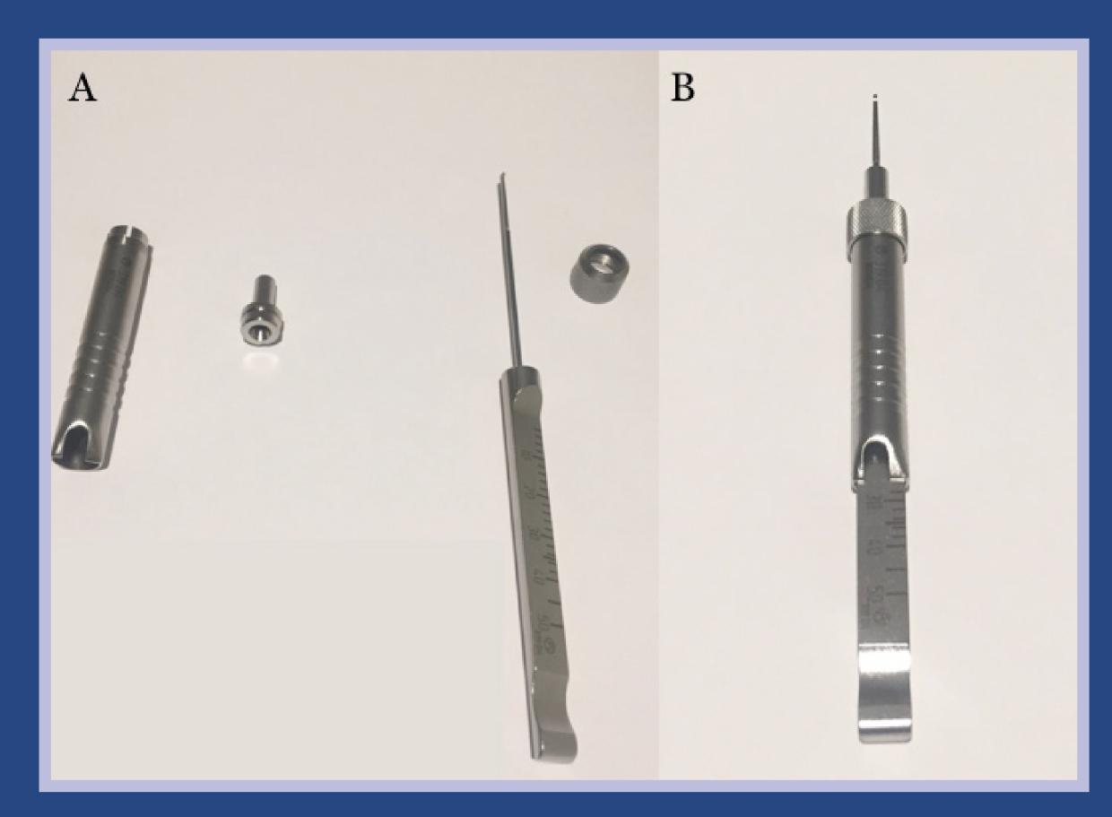
Figure 1: (A) The orthopaedic depth gauge disassembled. (B) An assembled depth gauge.
