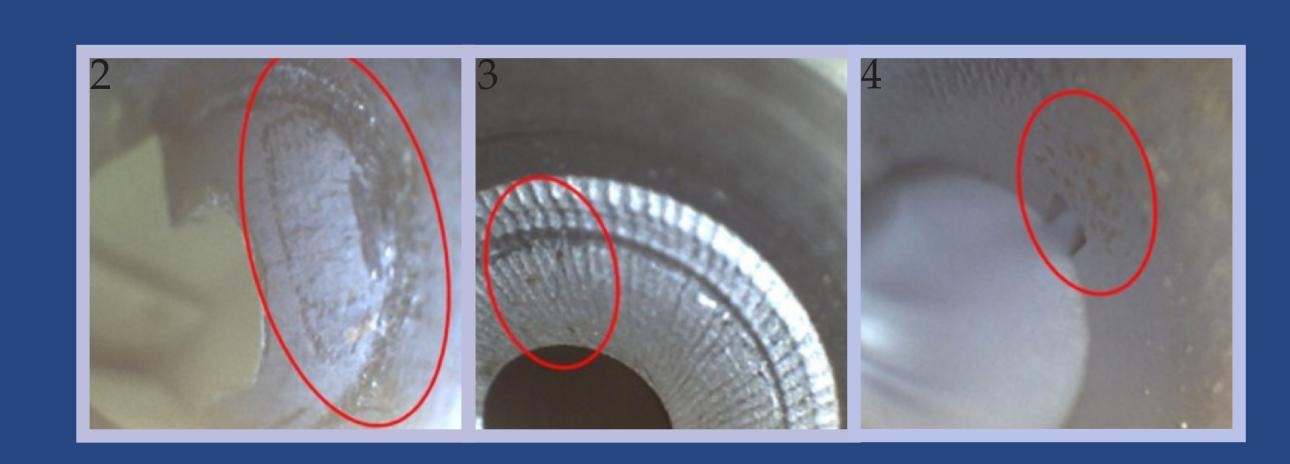
Figure 2: Debris within the large lumen of the device.
