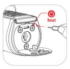
3. Find the hole where the reset button is located
