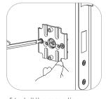
5.Install the mounting bracket and tighten the mounting bracket screws
