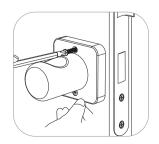
6.Install the rear panel handle and tighten the screws
