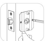
4.Install the mounting bracket and tighten the mounting bracket screws
