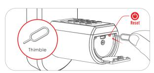
3. Find the hole where the reset button is located
