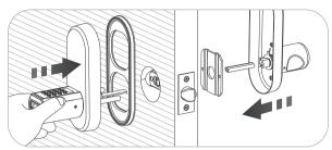
3. Insert the front handle toggle lever into the lock body
