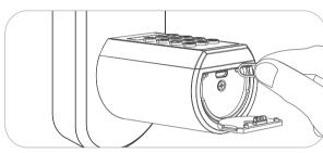
4.Insert the thimble into the hole and press the reset button
