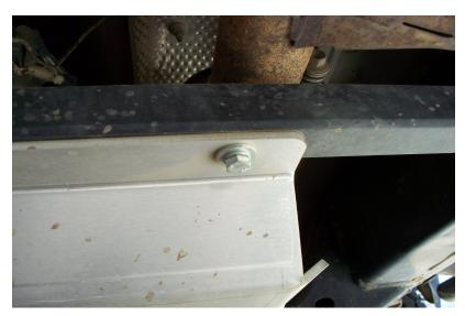
Step twelve: Install the cat protector tubes. The rock blocks and countersunk bolts fit in between the flanges of the protector tube. Align all skids and get all of the bolts for the protector tubes started. Leaving loose for now.
