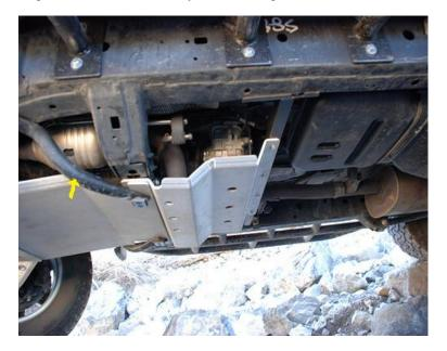
The protector tube is marked with the arrow. This picture also shows the rock blocks and how everything will be re assembled. You will re use the factory bolts on the opposite end of the rock blocks.
