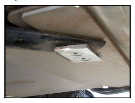
Step thirteen: Square up the cross member you installed earlier and tighten. You must do this before mounting the fuel tank skid, or you will not be able to get to the bolts.
