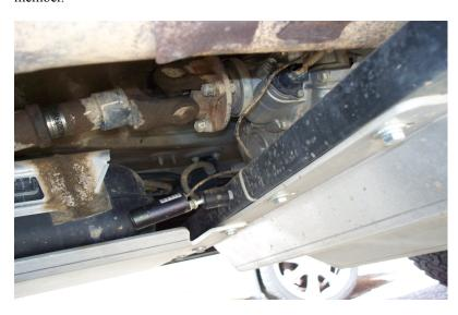
Square up and tighten all plates starting with the HD skid ,working your way back.
